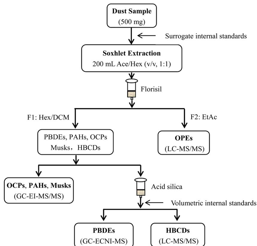
Fig. 1 Schematic representation of the dust sample preparation procedure.
