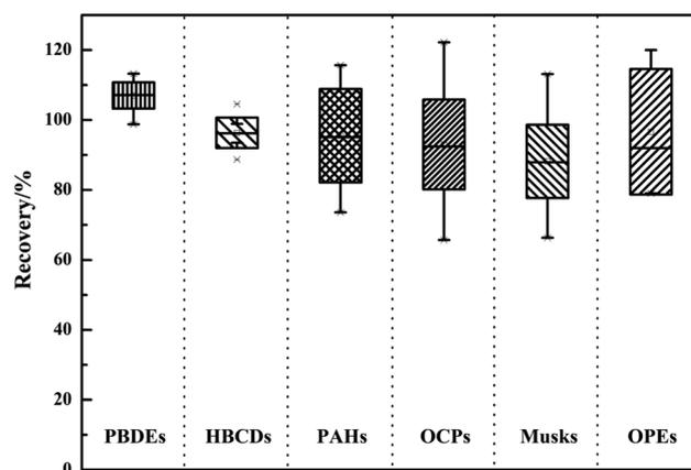
**Fig. 4** Box plots representing average recoveries ( $n = 9$ ) and relative standard deviations (RSD) for six classes of analytes under the optimized SPE method at three different concentration levels.
