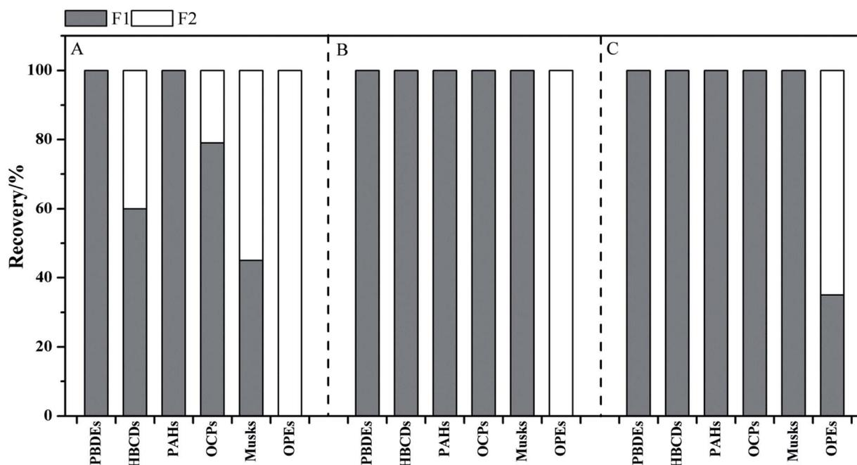
Fig. 2 The separation of PBDEs, HBCDs, PAHs, OCPs, Musks and OPEs on a 1 g/6 mL Florisil cartridge under three different elution conditions ((A) F1-10 mL Hex + F2-10 mL EtAc; (B) F1-10 mL Hex/DCM (v/v 8 : 2) + F2-10 mL EtAc; (C) F1-10 mL Hex/DCM (v/v 7 : 3) + F2-10 mL EtAc).
