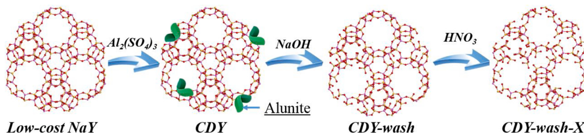
Scheme 1. Dealumination process for low-cost NaY zeolite.
