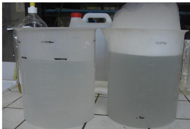
Fig. 7. The P3-ultrasil 10 solution before (left) and after (right) cleaning (shear stress = 16 Pa and time = 50 min).
