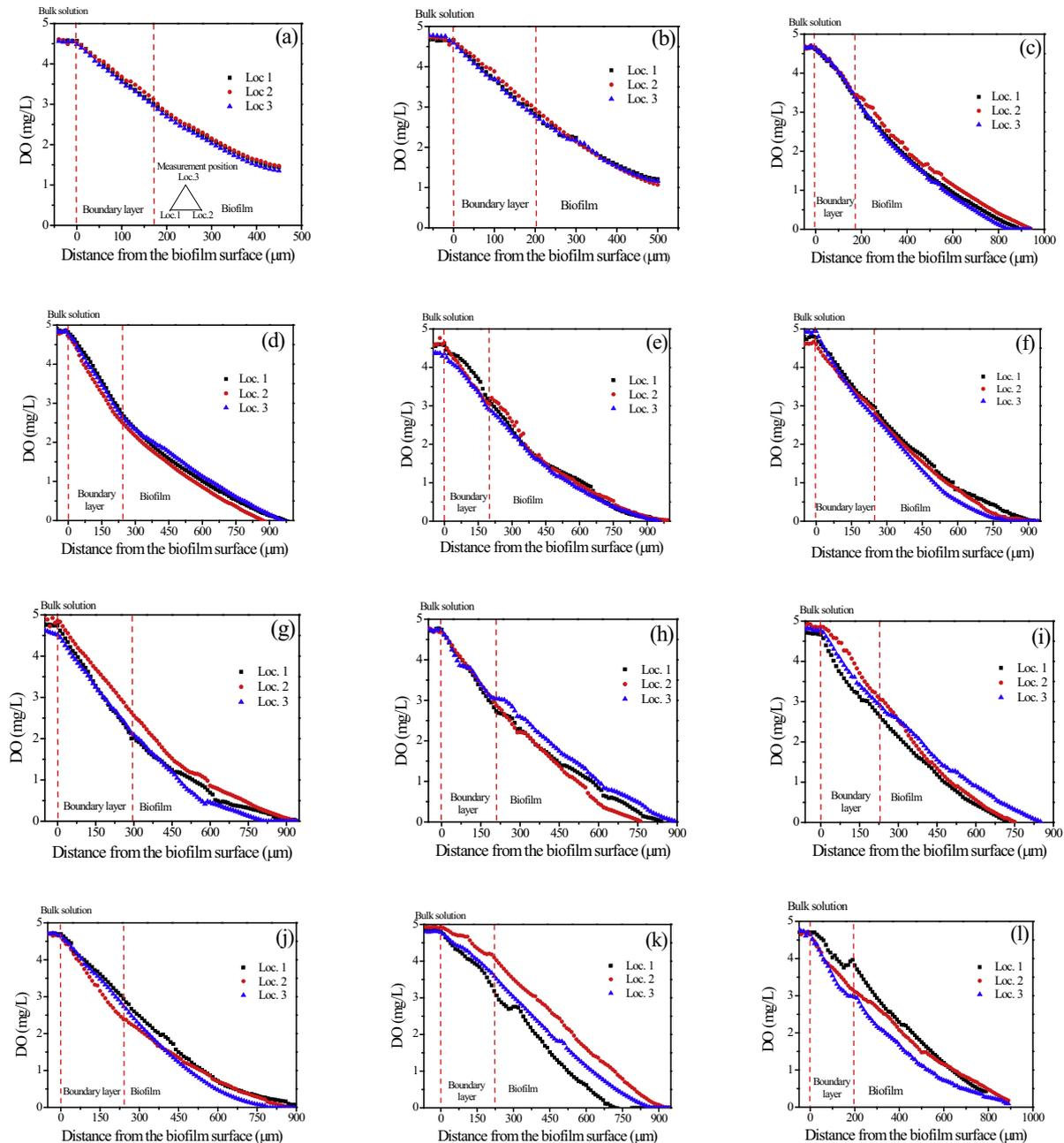
**Fig. 4.** DO profile within the biofilm at different time points: (a) 15 days; (b) 19 days; (c) 25 days; (d) 29 days; (e) 34 days; (f) 40 days; (g) 44 days; (h) 50 days; (i) 55 days; (j) 60 days; (k) 64 days; (l) 68 days.
