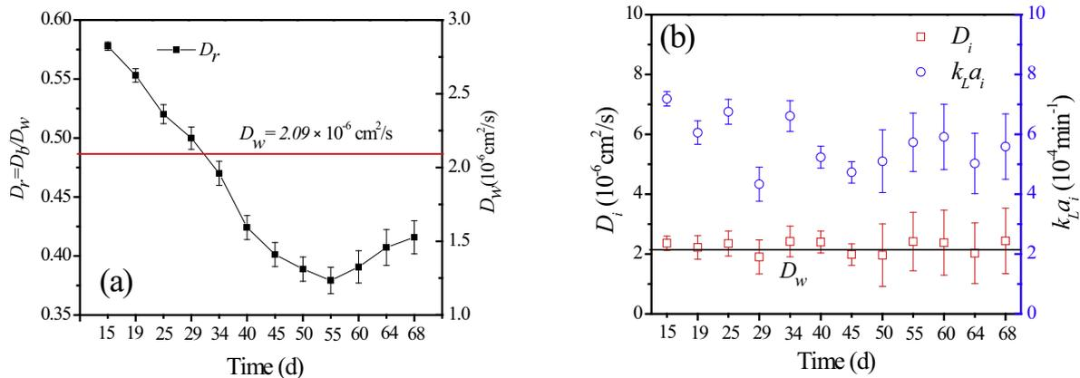
Fig. 6. Mass transfer of DO in the biofilm and boundary layer: (a) Variation of  $D_r$  in the biofilm; (b) Variation of  $D_i$  and  $k_La_i$  in the boundary layer.
