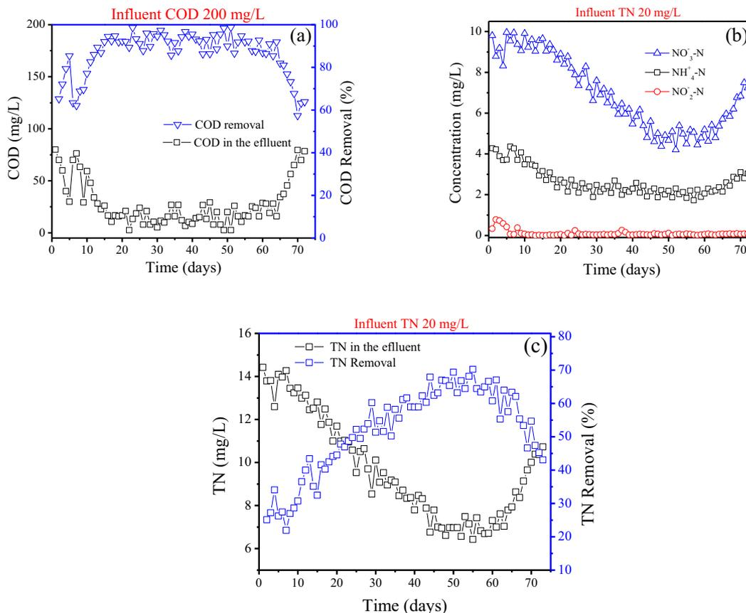
**Fig. 1.** Variation of oxygen-consuming substances: (a) the concentration of organics in the effluent and its removal efficiency; (b) the concentration of  $\text{NH}_4\text{-N}$ ,  $\text{NO}_2\text{-N}$  and  $\text{NO}_3\text{-N}$  in the effluent; (c) the concentration of TN in the effluent and its removal efficiency.
