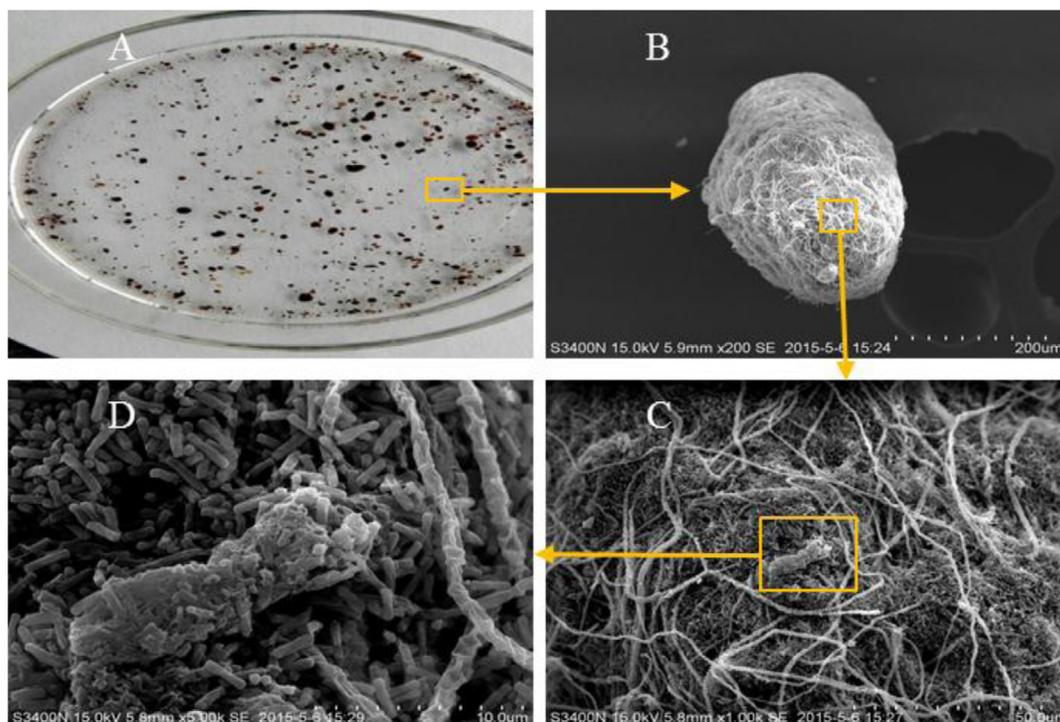
Fig. 5. Microscopic structure of the surface on granule sludge: (A) the photograph of GS; (B) the SEM image of GS ( $\times 200$ ); (C) the SEM image of GS ( $\times 5000$ ); (D) the SEM image of GS ( $\times 1000$ ).
