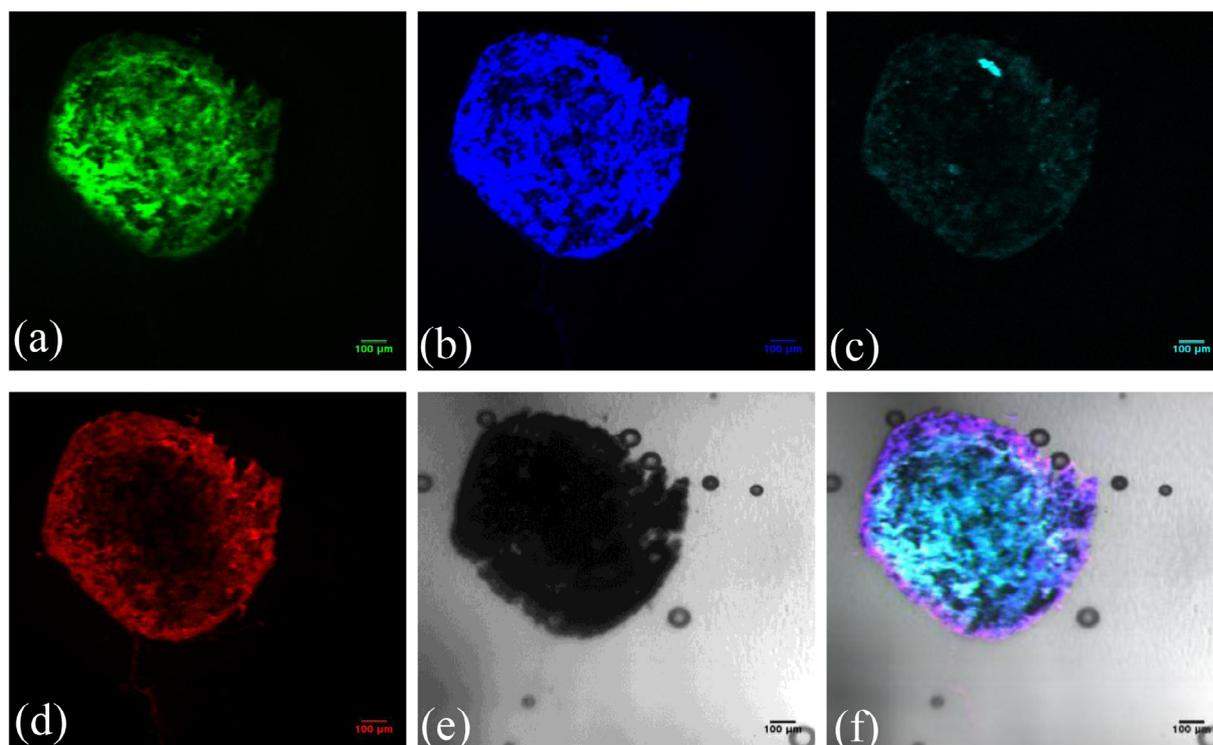
Fig. 7. EPS profile in a sludge granule: (a). CLSM image of proteins (FITC); (b). CLSM image of  $\beta$ -polysaccharides (Calcofluor white); (c). CLSM image of  $\alpha$ -polysaccharides (Con A); (d). CLSM image of lipids (Nile red); (e). Phase contrast photograph; (f). Combined image of individual images in (a)–(e).
