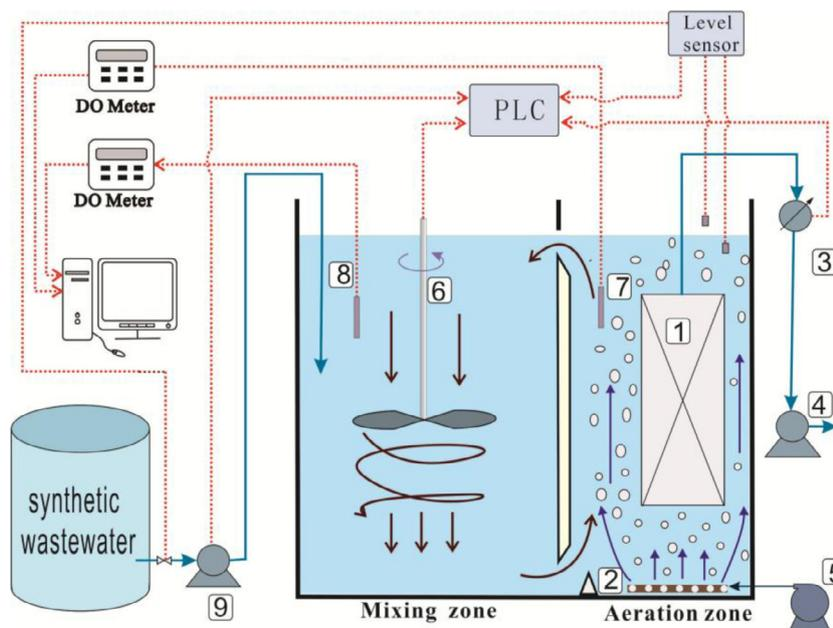
**Fig. 1.** Schematic diagram of the used MBR: (1). Membrane module; (2). Microporous aerator; (3). Vacuum meter; (4). Peristaltic pump of the effluent; (5). Air compressor; (6). Rotator; (7). DO probe in the aeration zone; (8). DO probe in the mixing zone; (9). Peristaltic pump of the influent.
