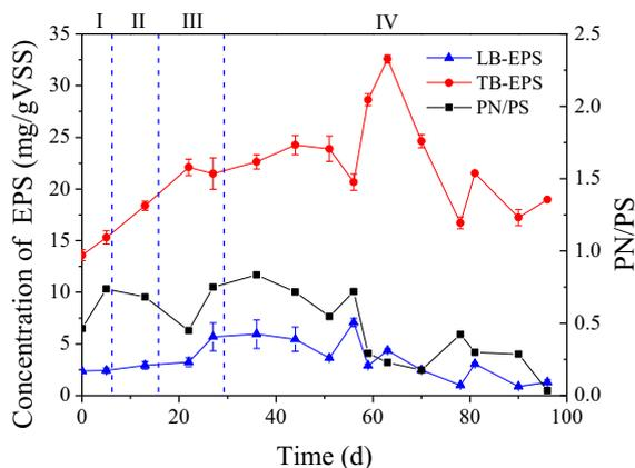
Fig. 6. EPS composition of granular sludge over time.
