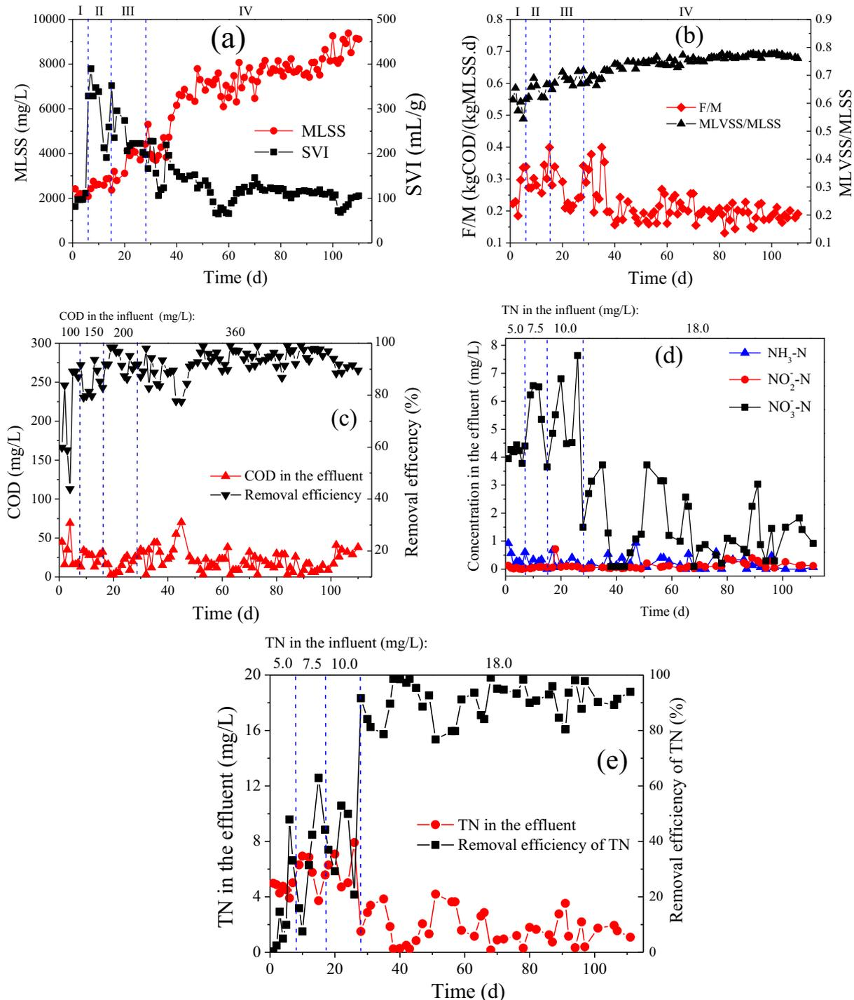
Fig. 2. Performance of the IC-MBR: (a). the growth of biomass and its settling ability; (b). the ratio of MLVSS/MLSS; (c). the removal of organic pollutants; (d). the concentration of  $\text{NH}_3$ -N,  $\text{NO}_2^-$ -N and  $\text{NO}_3^-$ -N in the effluent; (e). the removal of TN.
