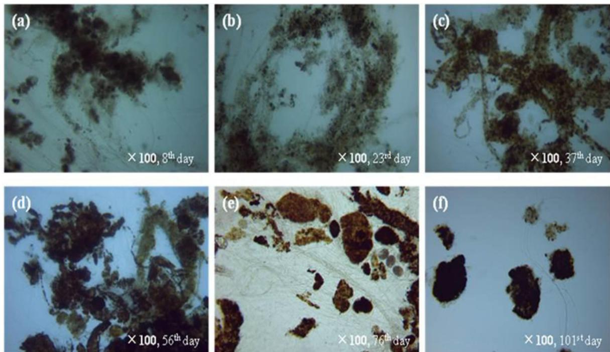
Fig. 3. Formation of granular sludge in the IC-MBR: (a)–(f) images of sludge granules on the 8th, 23rd, 37th, 56th, 76th and 101st day.
